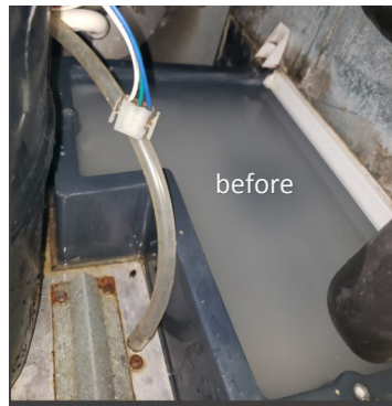
In some parts of the ice machine, limescale begins to come off.
